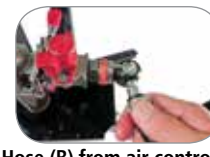
Hose (B) from air control to TOP air motor fitting. Connect exhaust hose (C—not shown) to BOTTOM air motor fitting.
