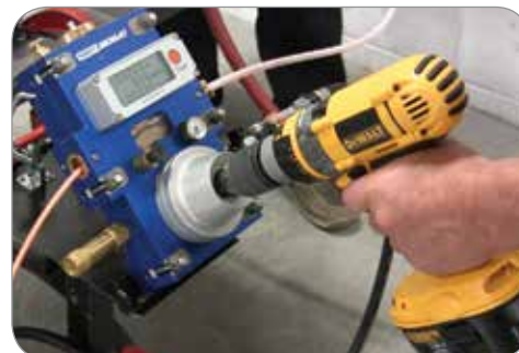
Hose (B) from air control to TOP air motor fitting. Connect exhaust hose (C—not shown) to BOTTOM air motor fitting.
