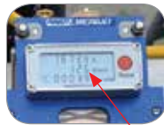
Adjust and maintain speed at 100-150 ft/min.
